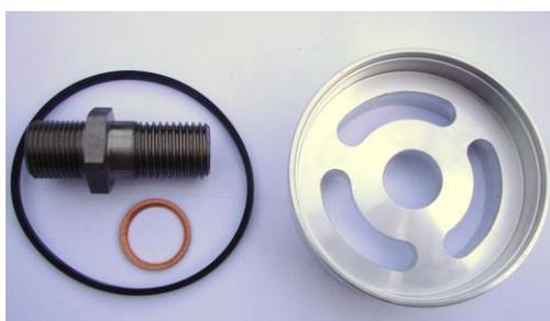
Remove the bolt, bowl, and old oil filter. Remove the large seal which sits in the groove in the filter head - it may be a tight fit. Remove the steel centre boss by placing a tommy-bar through the holes in the side and unscrewing it. Remove the splash plate (if fitted).
